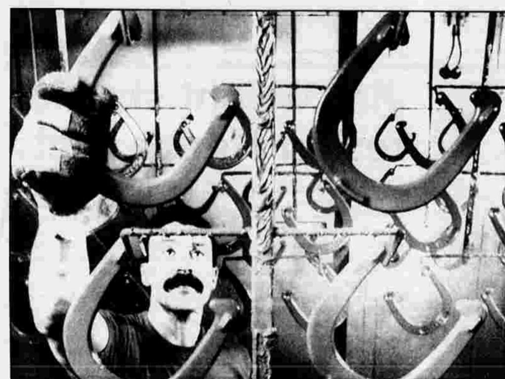
HORSESHOE MAKER — Raul Quinones, a production worker at the St. Pierre Manufacturing Co. of Worcester, Mass., removes a rack of horseshoes after their process through an electronic powder coating booth and curing oven Friday. St. Pierre is the world's largest horseshoe maker for the sport of horseshoe throwing, a sport now made popular by President George Bush.
